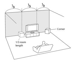
The placement of the SL-10S subwoofer can greatly affect the sound that is produces. In general, a good bass sound can be obtained by installing the subwoofer in a front corner, or at one-third the width of the wall, as shown. Experiment with different positions to find your listening preference.
